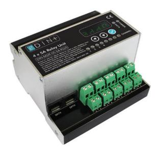
The Relay Contact Module is an ultra compact DIN rail mounted unit with connections for four relay outputs and an M-BUS network. Each feed through relay can switch 5A with a maximum module load of 20A.
