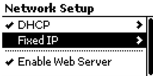
In the *Fixed IP* menu highlight *Use Fixed IP* and use the *Select* button to tick the option.
