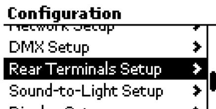
Each of the three terminals may be set as either a Contact Input or as an Analogue Output:
