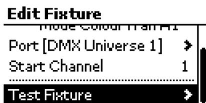
Press *Select* to show the current output levels of the DMX channels that the fixture is using.
