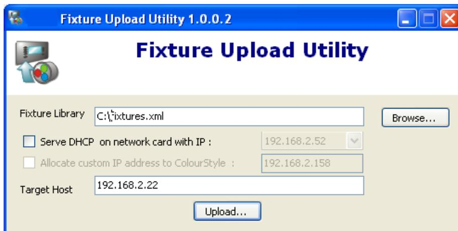
Browse for the location of the XML file, enter the IP address of the target ColourStyle, and click *Upload...* to transfer the file.
