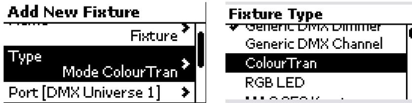
Scroll down to the fixture type that you want to use and press *Select* to tick that fixture.
