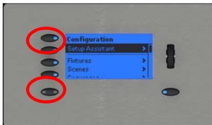
☞ Whilst holding the above, press and release the concealed *Reset* button.
