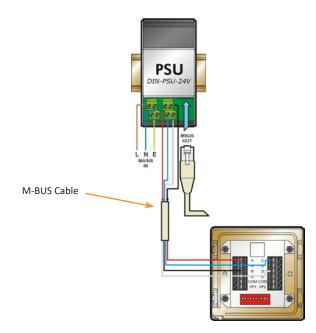
The M-BUS Cable may also be used other applications/separate systems including the Mode Tiger systems and DMX wiring.
