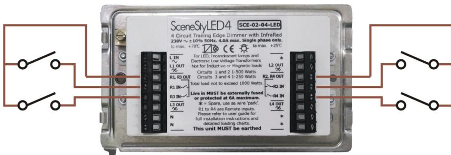
The remote switches are mains-live and therefore all switches and the cable to them must be mains rated.
