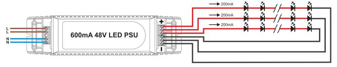
**IMPORTANT:** Each output MUST drive the same number of LEDs.
