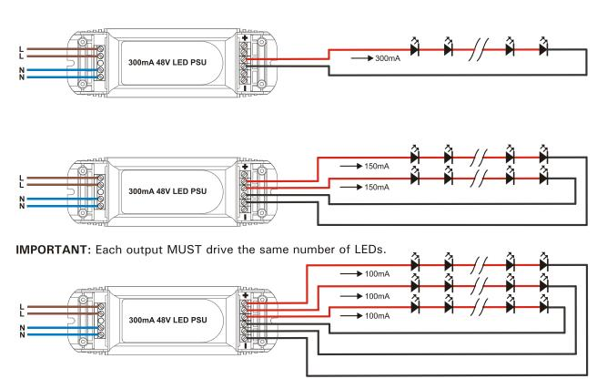
IMPORTANT: Each output MUST drive the same number of LEDs.
