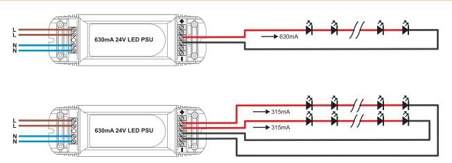
IMPORTANT: Each output MUST drive the same number of LEDs.
