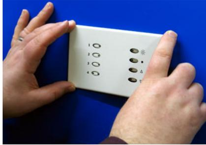
Firmly press the top right corner and then the bottom-right corner of the fascia until it clicks into place.
