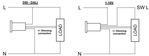
\* When used with digital dimming ballasts/drivers a permanent live supply is required.
