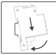
Modules must be installed within a suitable surface mount enclosure with integral DIN rail. Installation must be carried out by a qualified electrician in accordance with National Wiring Regulations and other applicable regulations. Compliance to EC EMC and Low Voltage Directives may be invalidated if not used or installed according to the published specification.
