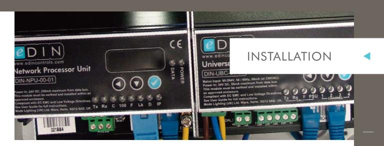
Compliance with the 17th Edition Installation Regulations is easily achieved including the use of MCBs and RCBOs on the input or output side of eDIN modules.
