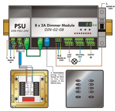
Each eDIN module incorporates an on-board, display driven, menu system through which circuit functions can be setup without the use of a computer. Depending on which modules are used, functions include dimming or switching operation, DALI address "Find" and group "Assign", maximum and minimum dimming levels, test modes and network diagnostics.
