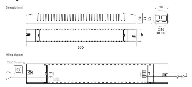
This product should be mounted in a well ventilated position and should not be covered by insulating materials. Installation should be in accordance with the relevant National Wiring Regulations and other applicable Regulations. Compliance with the UK and EC EMC and LV Directives may be invalidated if not used or installed according to the published specification.
