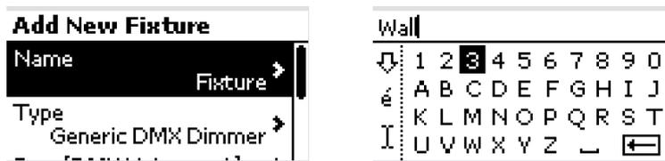
Give the fixture a name (this would normally be something descriptive about where the fixture is located, and what it's purpose is, for example "Wall Wash Left" or "Cove Colour Centre" etc.
