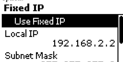
To set the IP address, use the scroll wheel to highlight *Local IP*
