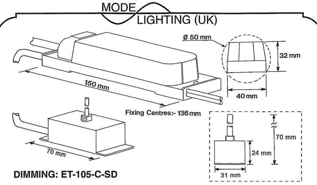
This self-dimmable model is designed to provide control of the lamp load between 10% and 100% through a pre-wired, boxed potentiometer with a 0.8 metre cable. If further remote dimming is required, only hard-fired dimmers should be used.
