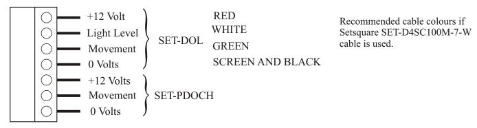
This diagram shows the connections for the SET-DOL sensor as shown in the Daylux SET-DDC installation Instructions.
