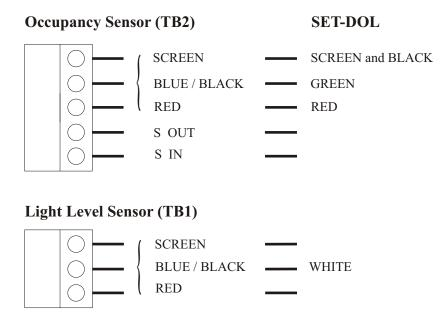
These diagrams show the connections to both TB1 and TB2 as shown in the Daylux II installation instructions and the changes necessary if using the SET-DOL sensor in place of an SET-ALD5 and a SET-PDOCH.
