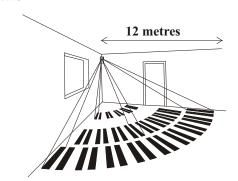
The output will be high when not detecting any Infra Red signal, and will go low when Infra Red detected.
