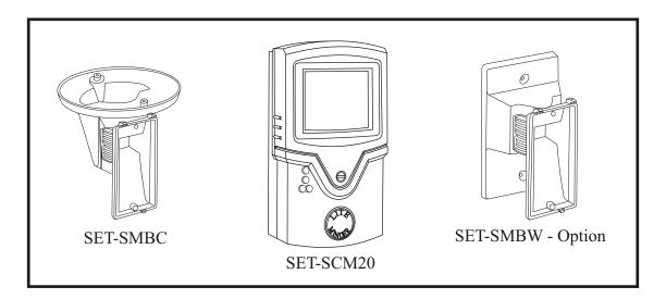
These instructions apply to the Liteminder SCM20-SMBC. Setsquare recommend all installations are carried out by a suitably qualified electrician and that these instructions are followed. Failure to do so may lead to damage to either the circuits or installer.
