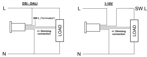
\* When used with digital dimming ballasts/drivers a permanent live supply is required. Terminate SW/L connection appropriately.
