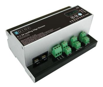
A four circuit Leading Edge mains Dimmer Module for the control of resistive and inductive lighting loads including compatible LED loads with the facility to select dimming or switched only operation of any circuit. A custom designed housing provides reliable power handling in a compact format.
